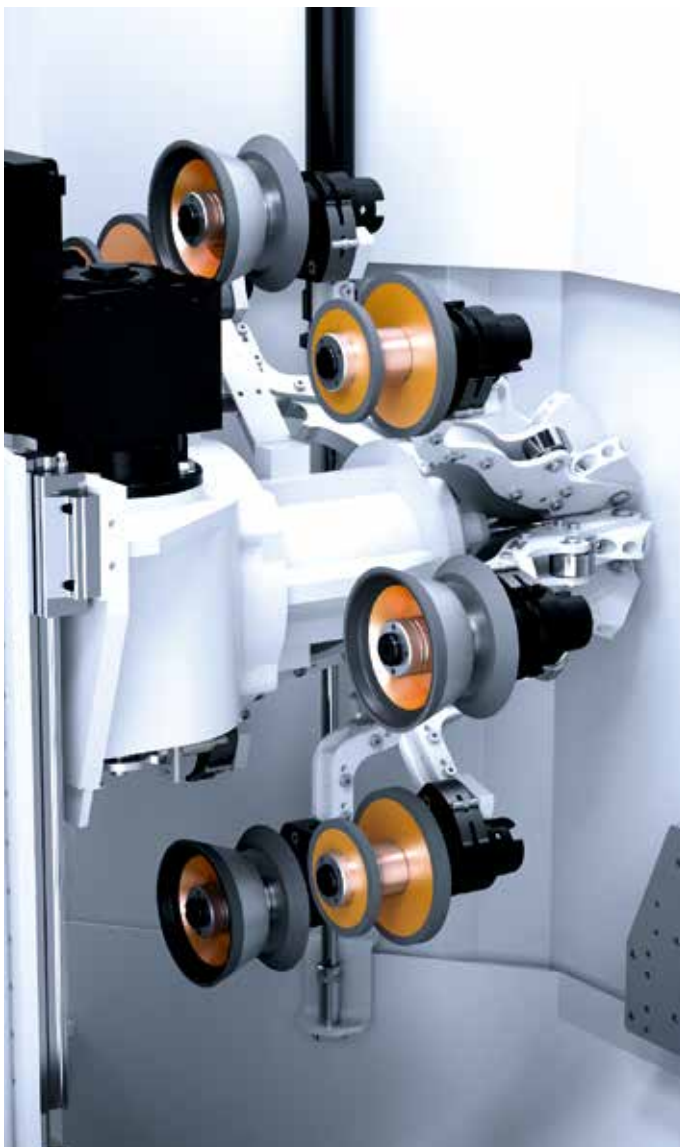
/// EIGHT-TOOL MAGAZINE for efficient tool changes and reduced non-productive time
