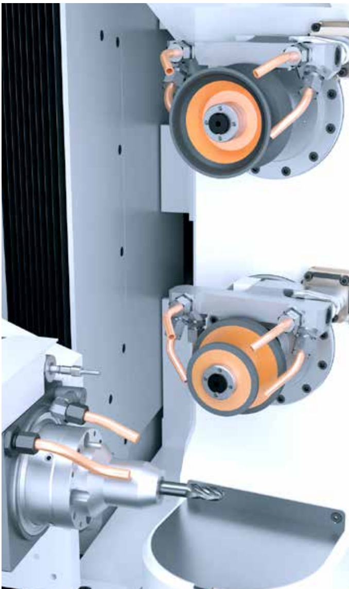
/// COOLANT NOZZLES for optimum coolant supply
