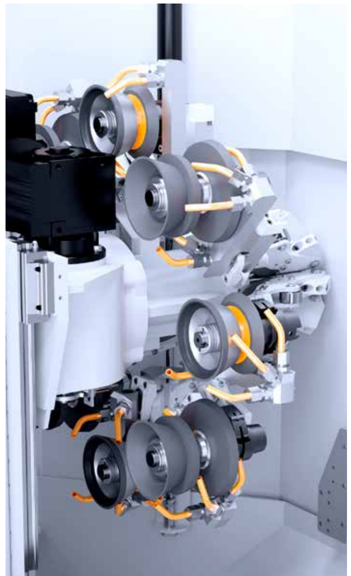
/// EIGHT-TOOL MAGAZINE including coolant nozzles
