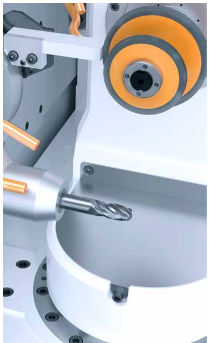
/// ROUGHENING UNIT for opening the abrasive wheel
