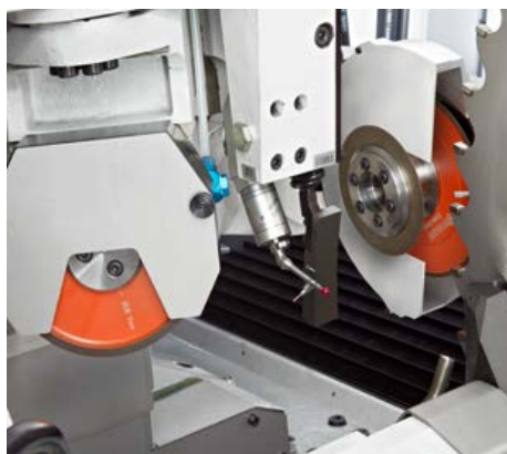
2 main spindles with up to 3 grinding wheels and the centrally situated measuring system.
