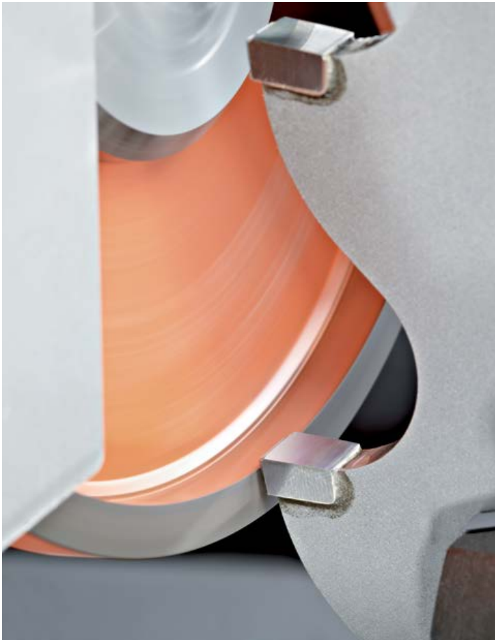
Tooth top machining.
