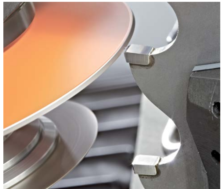
Grinding of negative face surface.
