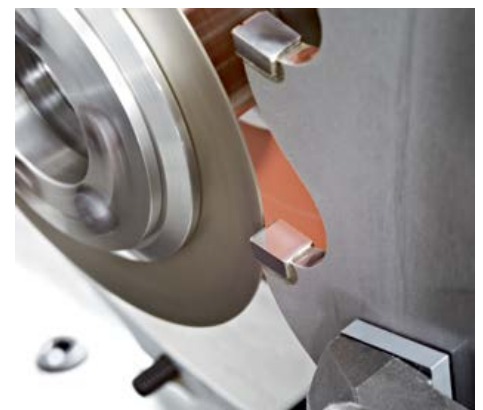
Grinding of chip breaker groove.
