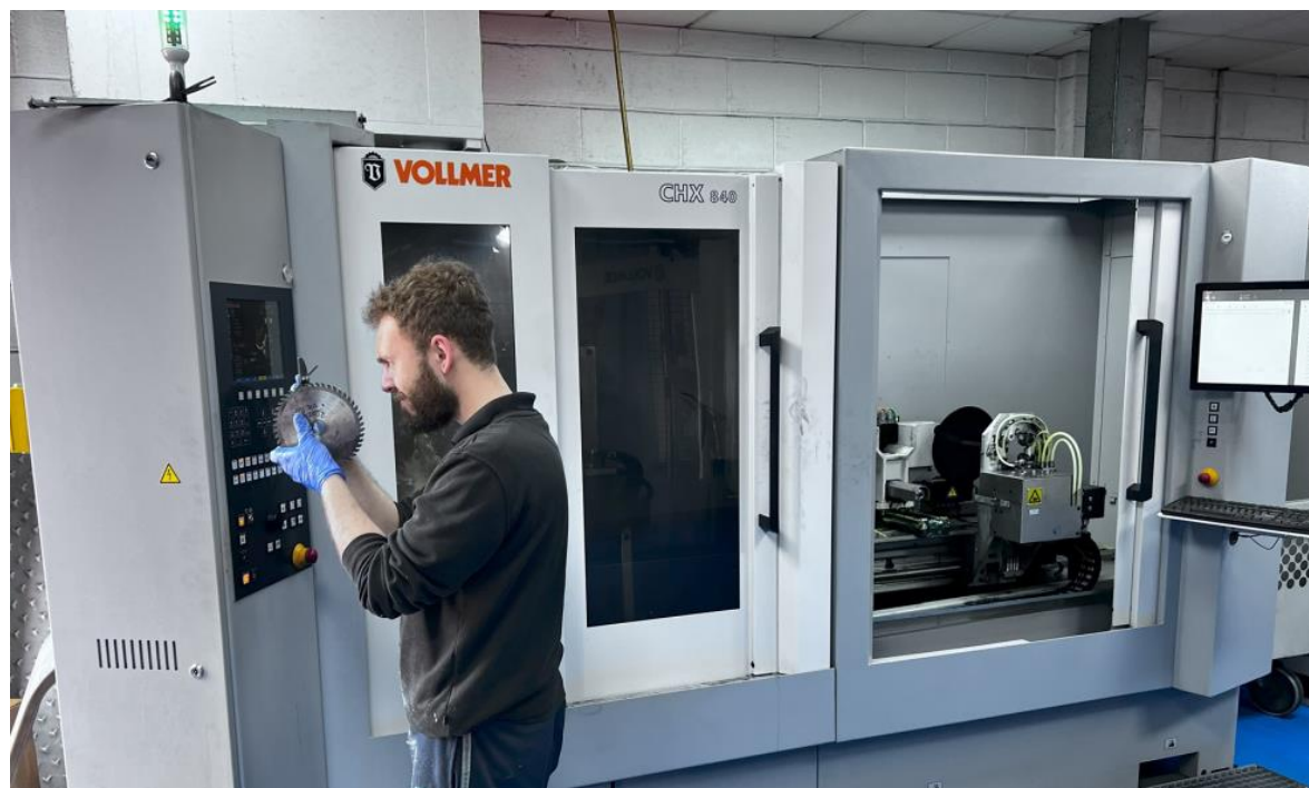
Caption: Several VOLLMER grinding machines from the CHD and CHX series ensure the precise sharpening of carbide-tipped circular saws at the southern English tool manufacturer Allied Tooling.
