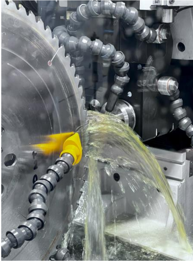
Caption: The VOLLMER QM eco select erosion machine is used by tool manufacturer Allied Tooling to sharpen its PCD-tipped circular saws for the UK.
