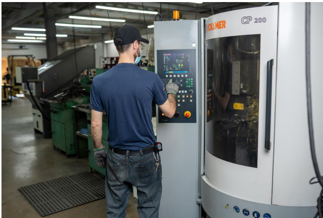
Caption: One of their VOLLMER machines is the CP 200 top and face grinder for carbide-tipped circular saw blades
