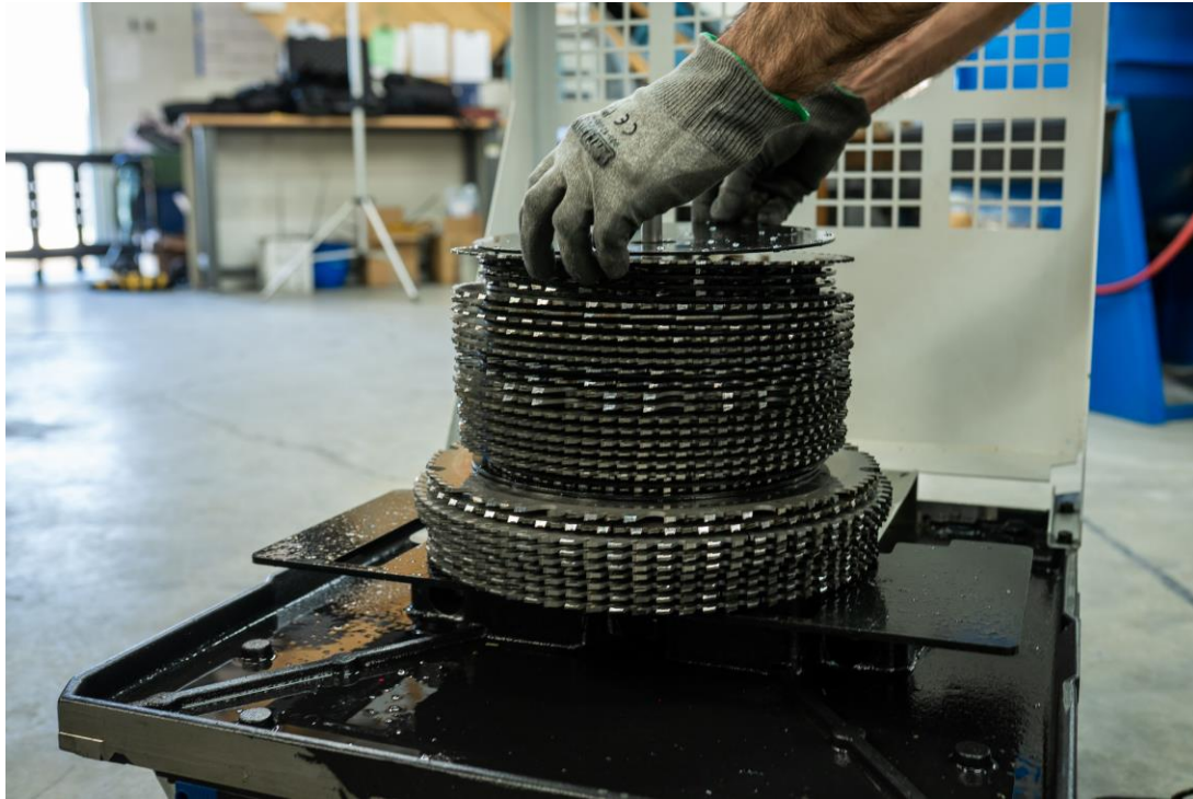
Caption: A stack of blades in one of the 5 carts of the VOLLMER ND 250 automation option
