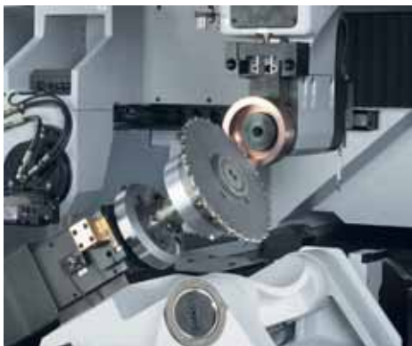
B1-axis (swivel range +/-30 degrees): eroding of a cutter with a cup disc
