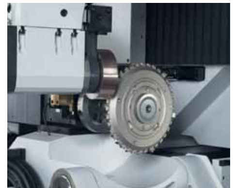
E1-axis in a swivelled position: eroding of a left-hand hogger
