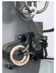
Tool magazine with 6 slots for eroding and grinding wheels
