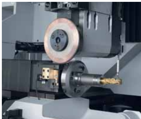
E1-axis (swivel range 330 degrees): gauging of a shank-type tool, right-hand as well as left-hand cutting, in a single setting
