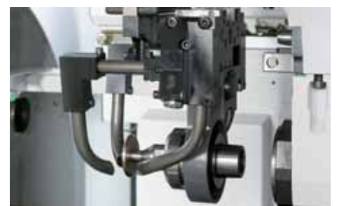
Eroding wheel with clamping cone HSK 63F and feeder device for dielectric fluid
