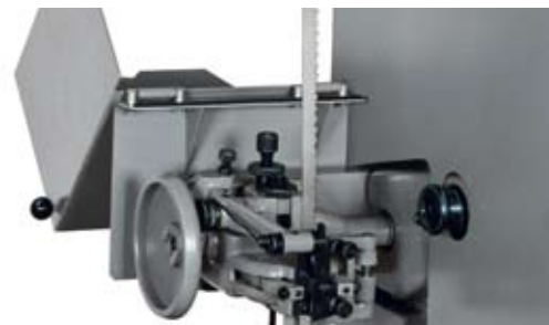
With a tooth setting attachment, band saw blades can be automatically set.
