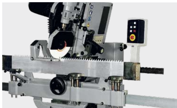
Clamping fixture with clamping carriage and indexing rail for gang saw blade widths of up to 220 mm
