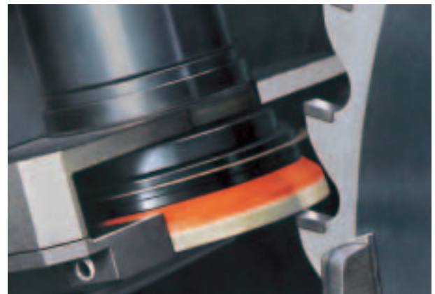
Cutting surface with negative hook angle
