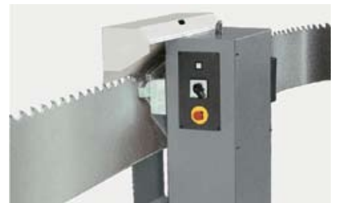
Synchronously driven auxiliary drive to assist band saw blade feed (optionally available)
