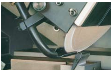
Automatic dressing of corundum grinding wheel (optionally available)
