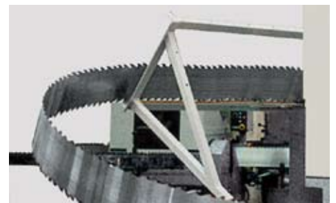
Loading bracket to simplify the insertion of big saw blades
