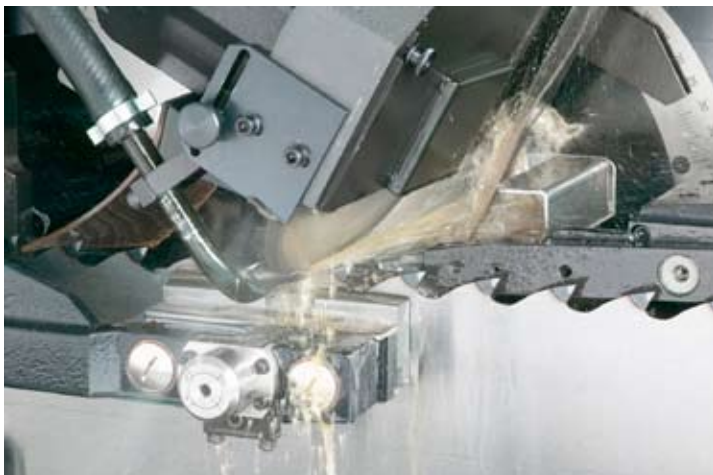
Oil cooling for long-lasting machines and less service application.
