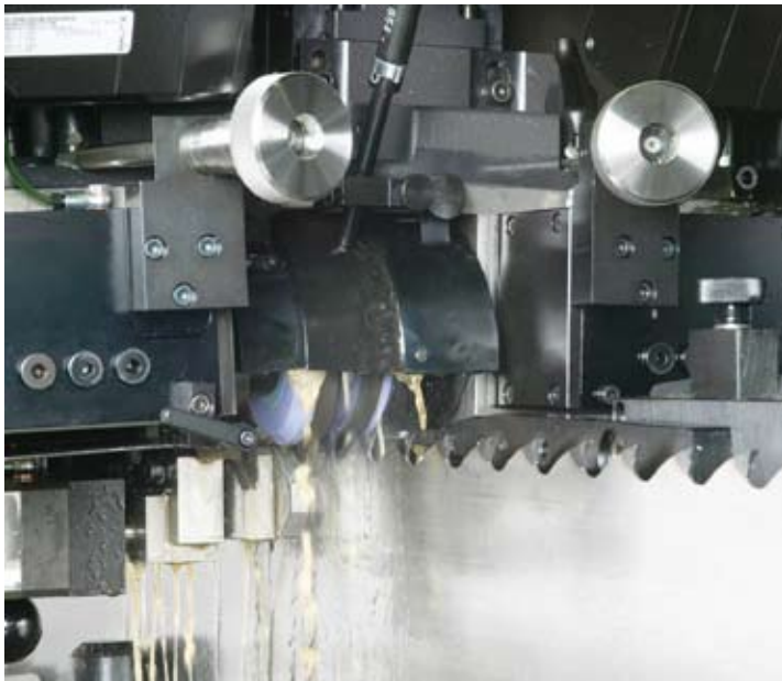
Oil cooling for long-lasting machines and less service application.
