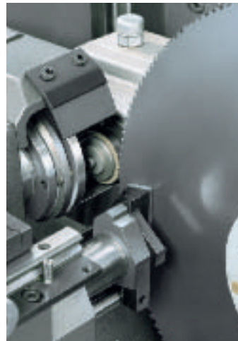
Grinding of chip breaker grooves in HSS saw blades with small tooth pitches from 4 mm
