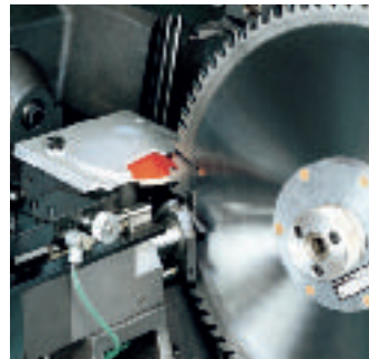
Sharpening the tooth face
