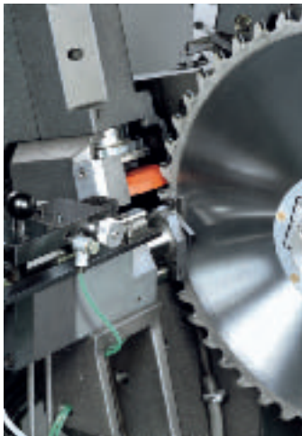
For tooth shapes with negative hook angles of up to 30°
