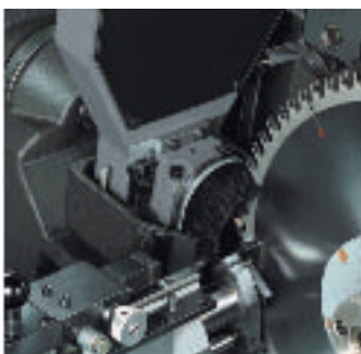
Hollow face grinding device as optional extra
