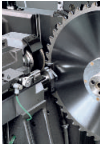
Grinding of chip breaker grooves in carbide-tipped circular saw blades
