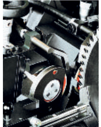
Measuring device for compensation of grinding wheel wear on request
