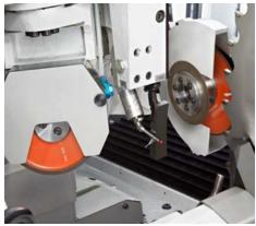
2 main spindles with up to 3 grinding wheels and the centrally situated measuring system.
