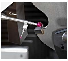
The measuring probe, which is standard within the machine, takes all relevant parameters such as cutting width, width of saw blade body and hook angle.
