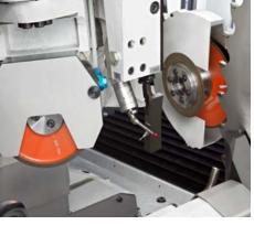
Grinding of chip breaker groove.
