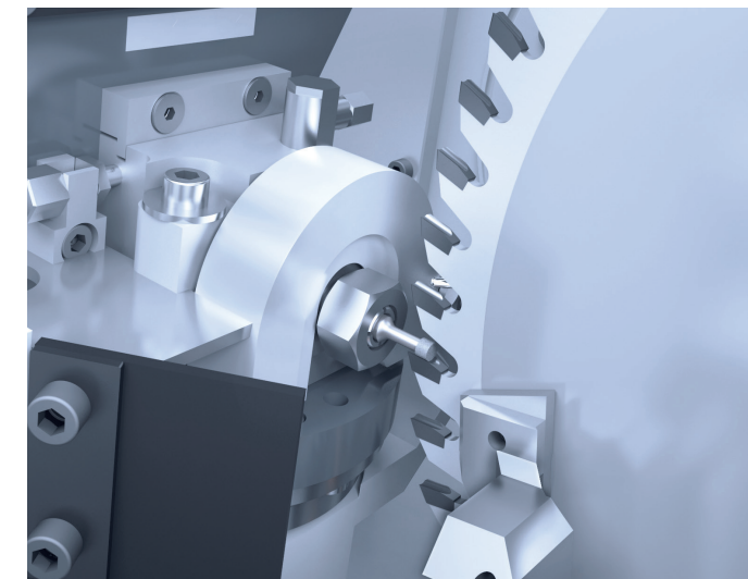
/// HOLLOW FACE MACHINING for excellent results in furniture manufacture
