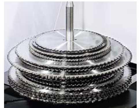
Up to 50 carbide-tipped saw blades of various diameters and tooth geometries can be stacked on each of the loading carriages.
