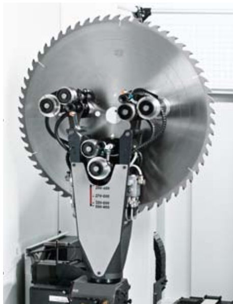
A standard gripper for the ND 320/340/360, designed for the automated machining of saw blades of up to 840 mm in diameter and weighing up to 20 kg.
