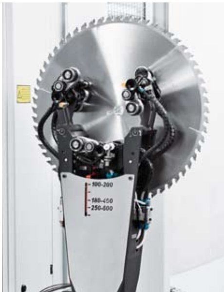
A standard gripper for the ND 230/250/270, designed for the automated machining of saw blades of up to 630 mm in diameter.
