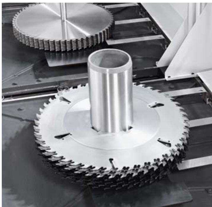
Saw blade stacks on the ND 320/340/360 loading carriage.
