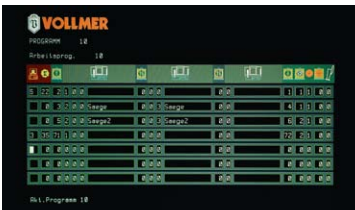
You can program various saw blade stacks on the loading system regardless of the data input station.
