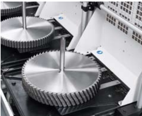
A loading carriage with a single saw blade stack in a productive operation mode.
